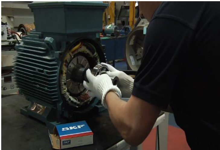
Correct bearing fitting methods and procedures to ensure long motor life
