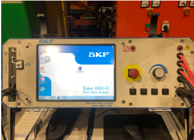
Surge comparison testing to ensure winding integrity
