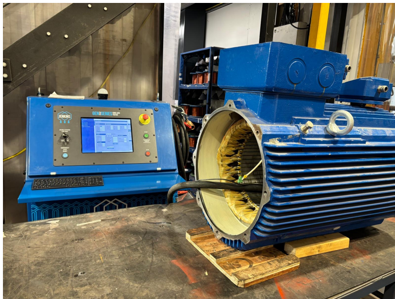
Core loss testing to prove stator core condition and verify motor efficiency pre and & post rewind
