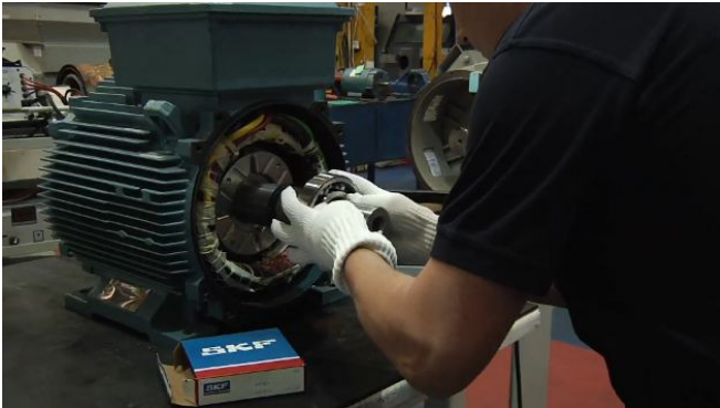
Correct bearing fitting methods and procedures to ensure long motor life
